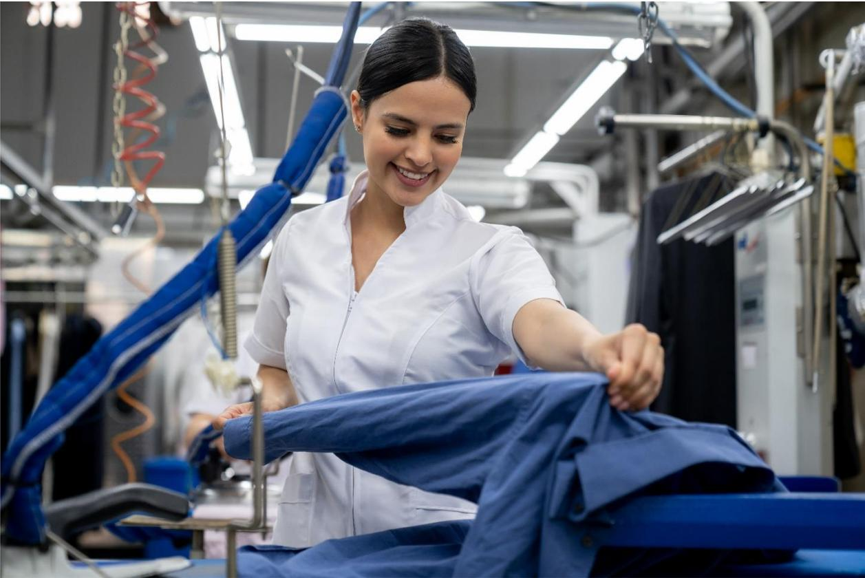
All the stitched garments are finished prior to sending a shipment to customers. Finishing means removing all creases and wrinkle from the garment, cleaning dusts and loose threads and repairing defective pieces.
