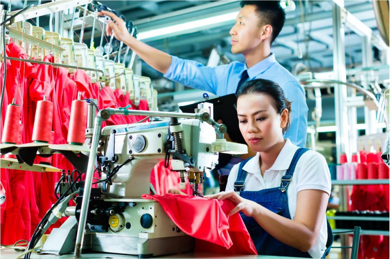
After fabric cutting and printing process (optional process), cut components are sent to the sewing department. Sewing operators stitch and assemble garment components one by one and make the complete garment.
